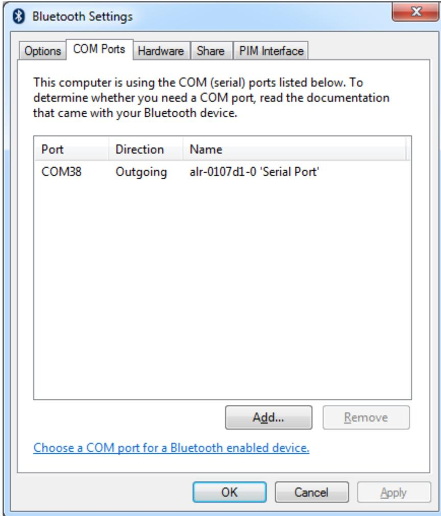
Open the serial terminal software (e.g.TeraTerm) and select the Bluetooth COM port:
